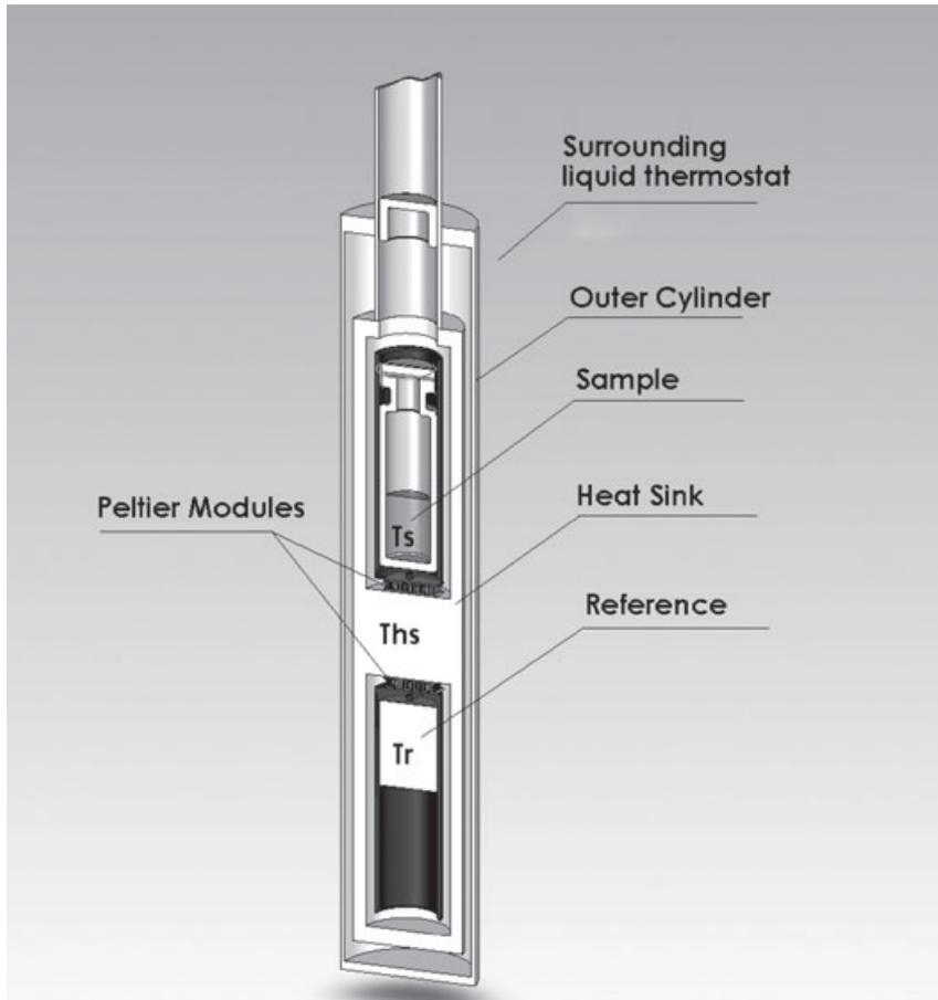
**Fig. 1.** Temperature differences between the sample ( $T_s$ ) and a thermally inert reference ( $T_r$ ) is continuously measured in a heat sink ( $T_{hs}$ ). The detection limit of the instrument expressed by the manufacturer is  $\pm 0.225 \mu\text{W}$ . Figure courtesy of Thermometric/TA Instruments, Jarfalla, Sweden.
