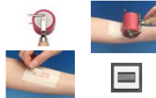
Fig. 4 The tape stripping area of the skin is defined by a template. Tapes are pressed on the skin by a roller (pressure of 140 g/cm 2 ) and fixed on a slide frame.
